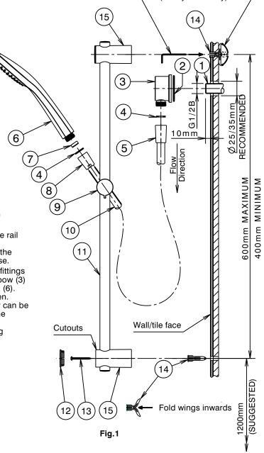
Use a small allen key or nail to spread wings of anchor behind wall
