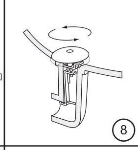
ROTATE ASSEMBLY 90 DEGREES AND ENSURE HOOK ENGAGES INTO WASTE
